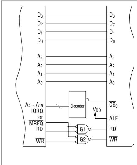
**Note:** Select either IORQ or MREQ so that the Z80 switching characteristics determined by the crystal oscillator for the Z80 match those of the IC described in this data sheet.
