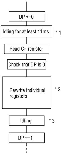
\*1 Time until the DP bit becomes 0 under assumption that oscillation is in progress.
