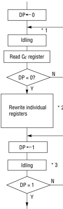
\*1 Processing by other IC or wait time to prevent unnecessary readouts which occur frequently. A measure is 1 ms.
