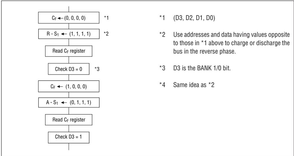
(b) Checking oscillation using software
