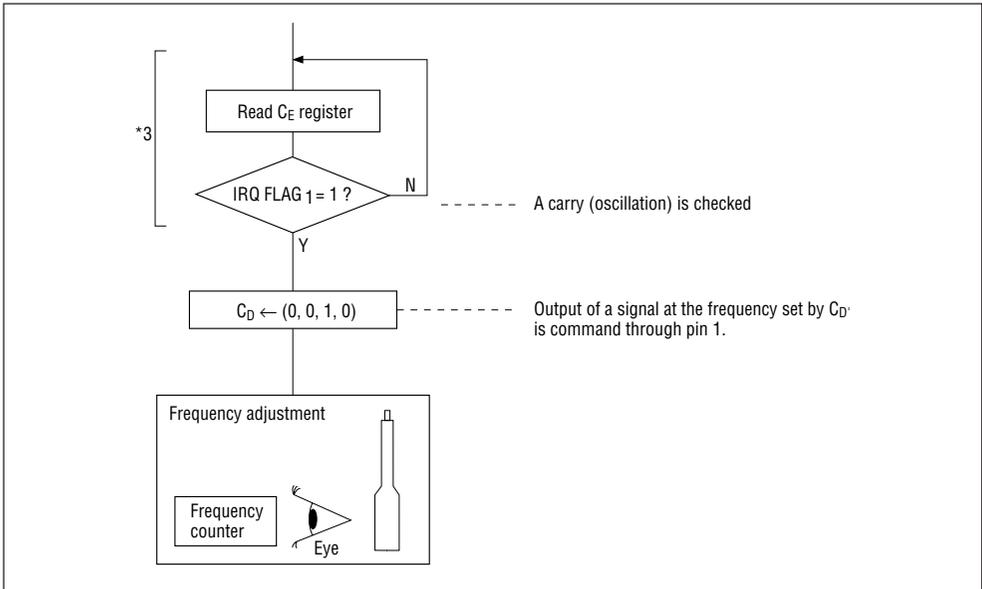
\*1 To cancel data protection, oscillation must be in progress. It takes about 13 ms (2 ms during which the writing of  $DP \leftarrow 0$  is inhibit in the rising of  $CS_1$ , plus 11 ms required until  $DP = 0$  is executed.) This loop includes a wait time before oscillation starts. Usually, the loop takes 0.5 to 2 seconds. When the power is turned on, the value of the DP bit is unpredictable. When the value is 0 incidentally, the loop does not return.
