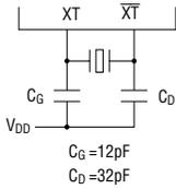
Crystal oscillator: P3 manufactured by Kinseki Co., Ltd.
