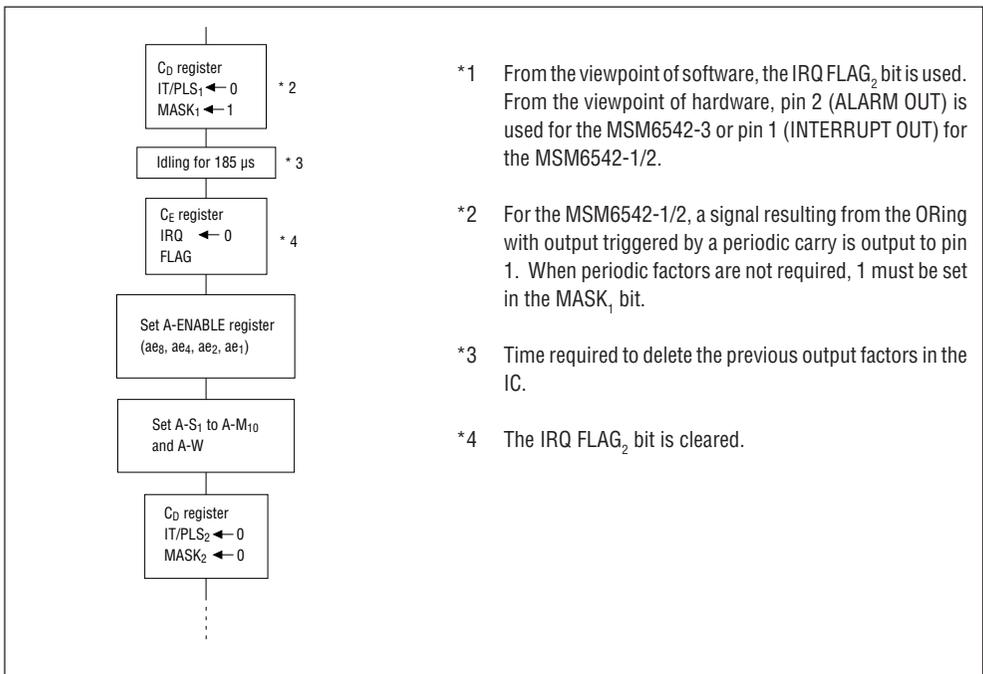
\*1 From the viewpoint of software, the IRQ FLAG<sub>2</sub> bit is used. From the viewpoint of hardware, pin 2 (ALARM OUT) is used for the MSM6542-3 or pin 1 (INTERRUPT OUT) for the MSM6542-1/2.
