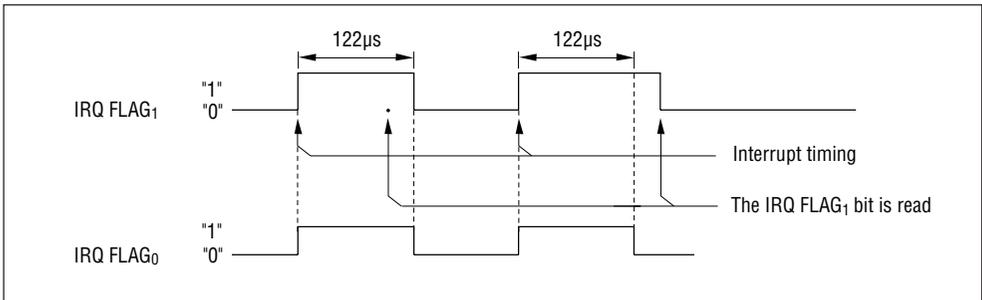
**Note:** When the IRQ FLAG<sub>1</sub> bit is read within the 122 µs interval with the MASK<sub>1</sub> bit set at 1, it is not cleared. The IRQ FLAG<sub>1</sub> bit is cleared after the 122 µs interval ends.
