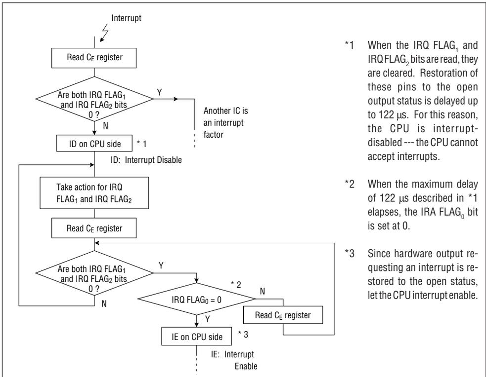
\*1 When the IRQ FLAG<sub>1</sub> and IRQ FLAG<sub>2</sub> bits are read, they are cleared. Restoration of these pins to the open output status is delayed up to 122 μs. For this reason, the CPU is interrupt-disabled --- the CPU cannot accept interrupts.
