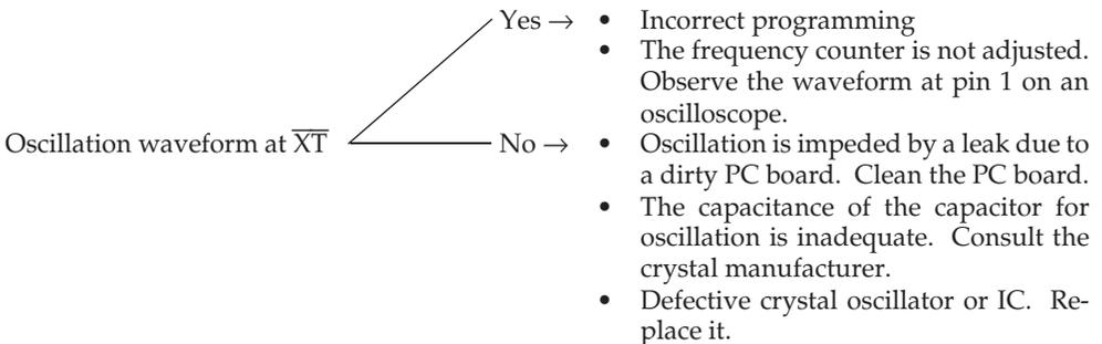
Possible causes when the loop marked \*1 or \*3 takes a long time (2 or 3 seconds or more)
