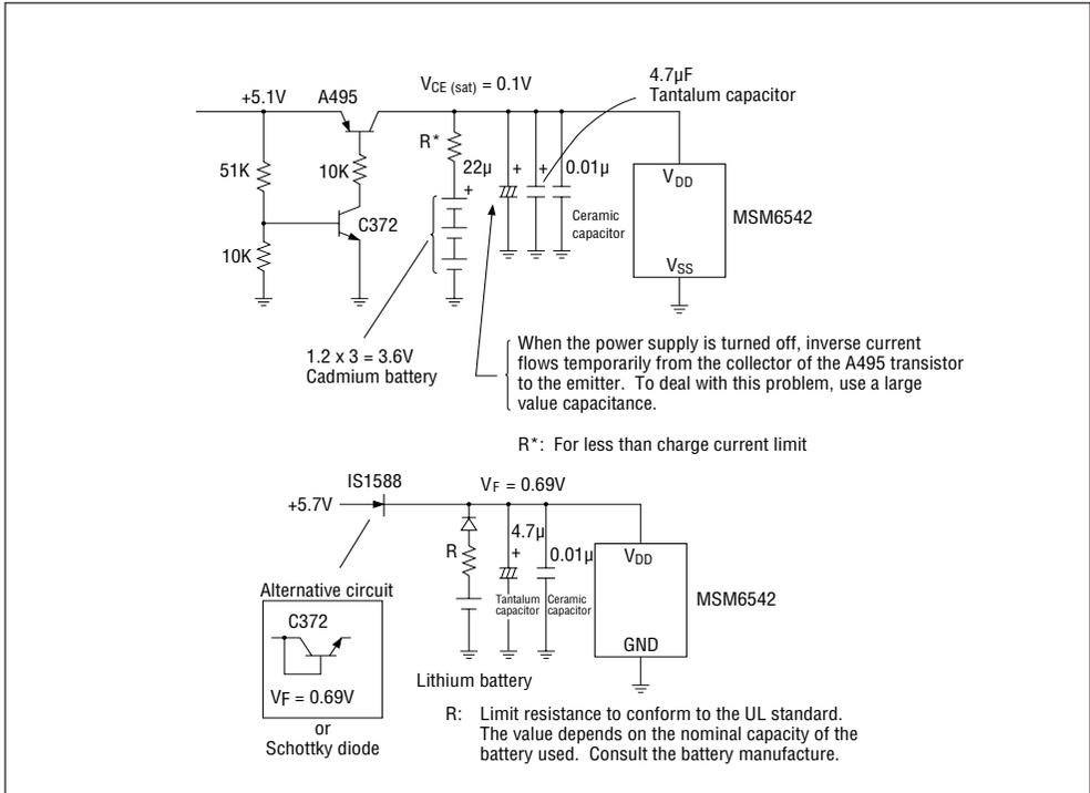
Sample main power supply monitor circuit
