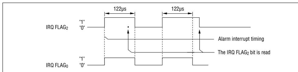
**Note:** When the IRQ FLAG<sub>2</sub> bit is read within the 122 μs interval with the MASK<sub>1</sub> bit set at 1, it is not cleared. The IRQ FLAG<sub>2</sub> bit is cleared after the 122 μs interval ends.
