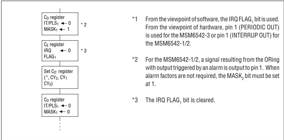
\*1 From the viewpoint of software, the IRQ FLAG<sub>1</sub> bit is used. From the viewpoint of hardware, pin 1 (PERIODIC OUT) is used for the MSM6542-3 or pin 1 (INTERRUPT OUT) for the MSM6542-1/2.
