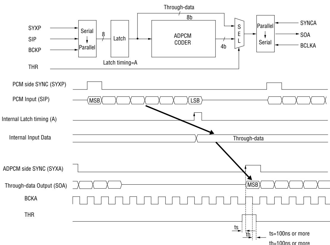
Note: That data-ship may occur when the rising edge (data load point) of SYXA and input of the internal latch timing overlap each other.
