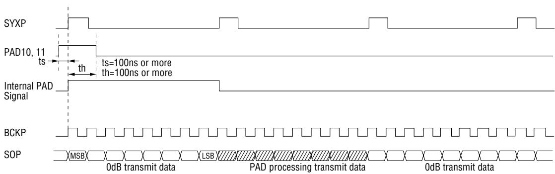
As mentioned above, PAD and MUTE processings are performed according to the rising edge of SYXA. Even if BLOCK is not 128 kHz, these processings are performed in the absolute time counted from the rising edge of SYXA.
