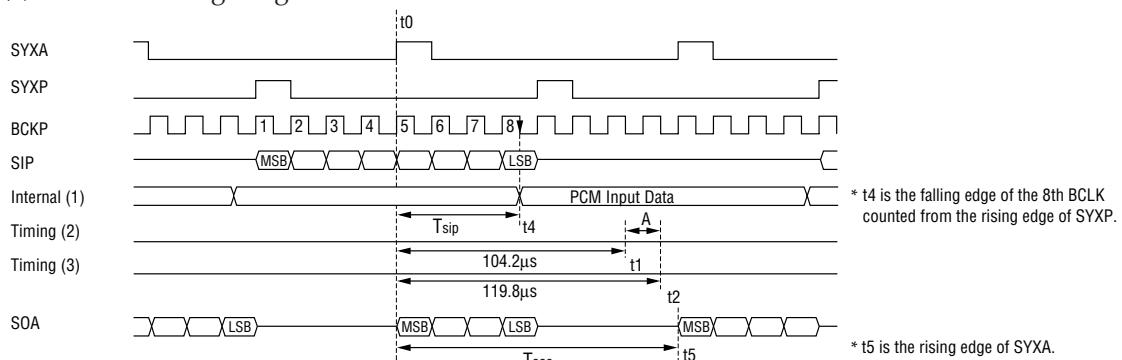
(b) DECODER Timing Diagram
