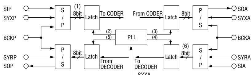
In this device, internal operating signals are generated according to the ADPCM side SYNC (SYXA) signal.
