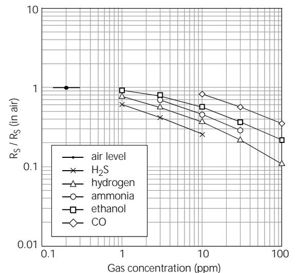
Fig 3. Sensitivity characteristics
