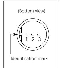
Fig 1c. Pin Layout
