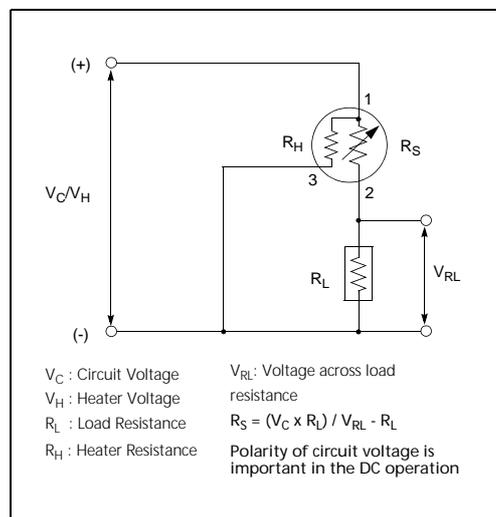
Fig 2. Standard circuit
