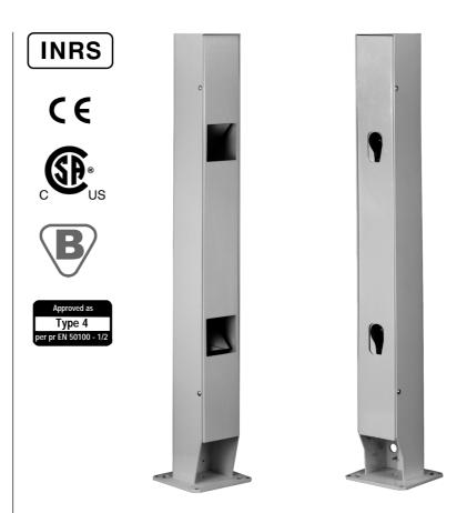
The FF-SPS4 access control systems are protective equipment designed for the control of dangerous zones in Industry. The intrusion of a person inside the zone is detected by the interruption of one or several infrared beams permanently selfchecked by an electronic circuitry which outputs an alarm signal toward the machine control circuitry. The opening of the output contacts due to the detection immediately stops the dangerous movement.
