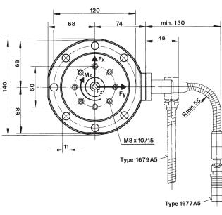
Fig. 1: Dimensions Dynamometer Type 9272
