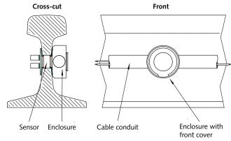
Fig. 2: Sensor assembly with conduit
