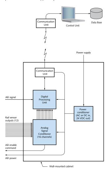
Fig. 1: Block diagram of Rail WIM system
