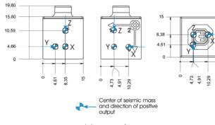
Fig. 3: Dimensions and directions of action
