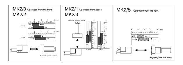
The MK2/2 and 2/3 are available as Form A and Form B sensors. The standard cable is a 4-wire round - core 4 x  $0.14~\text{mm}^2$  (cable sheath and wires are white) forming a sabotage loop. See example of this loop to the right.
