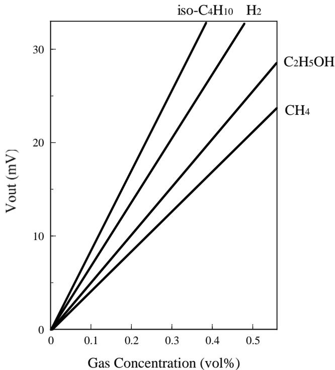
The graph opposite shows the relative sensitivity characteristics for the flammable gases Methane, Iso-Butane, Hydrogen and Ethanol.
