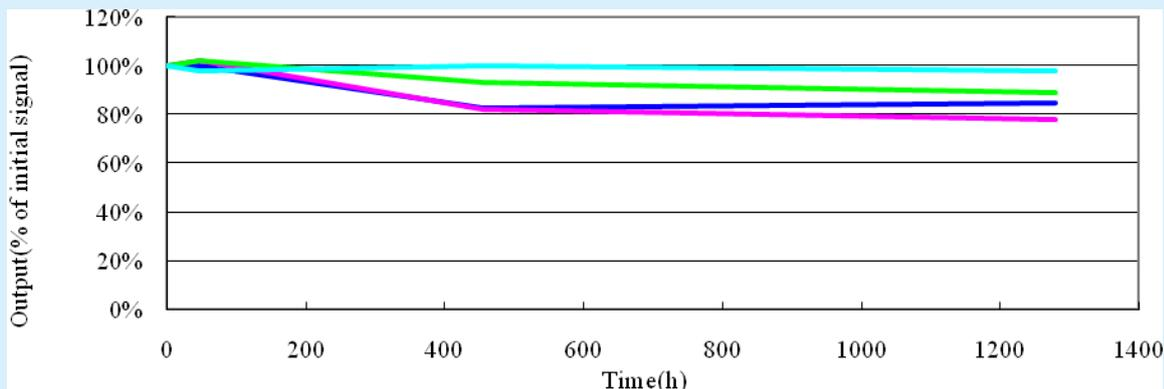
Fig. 8 : Durability in high temperature (50 degree C) and high humidity (90%RH)
