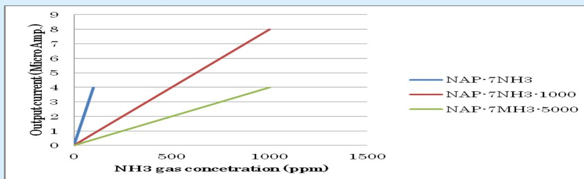
Fig.2 : Gas Sensitivity of NE4-NH3 series
