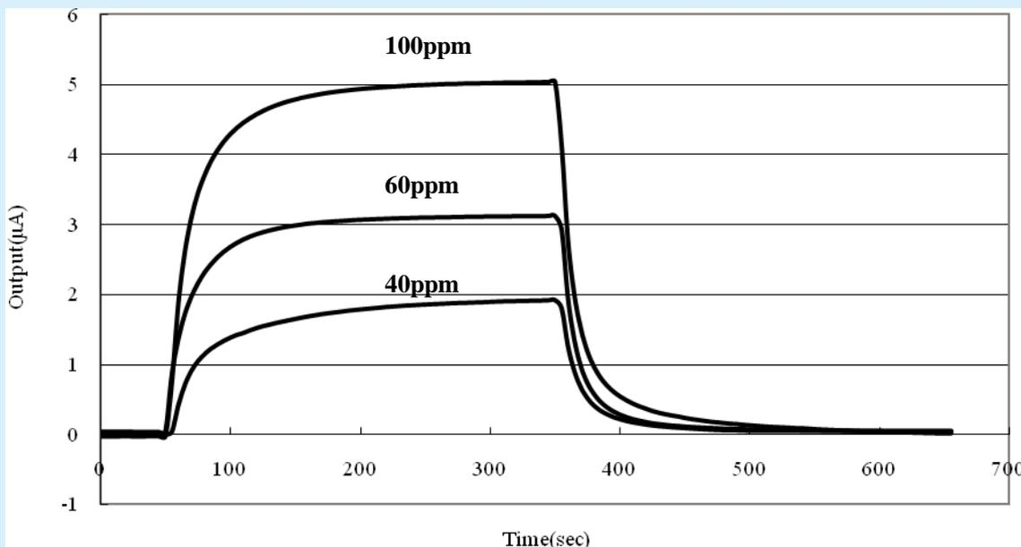
Fig.4 : Response and recovery characteristics
