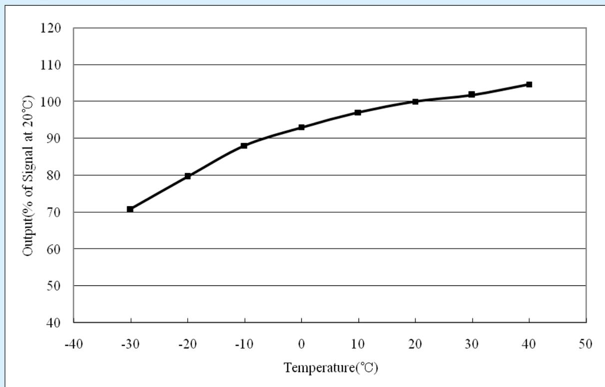
Fig. 3 : Typical temperature coefficient of NE4-NH3
