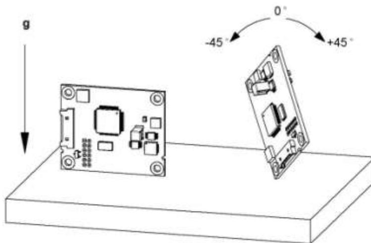
Figure 5-2: Accelerometer Calibration Starting Orientations
