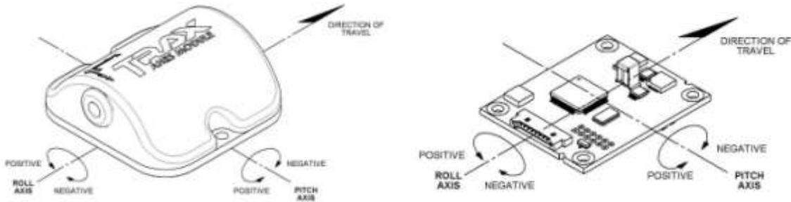
Figure 4-1: Positive & Negative Roll and Pitch Definition
