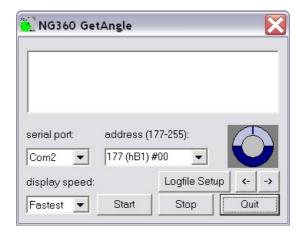
If more than one sensor is connected to the same bus, the address 177 (hB1) #00 (as in the figure above) must not be used!!!
