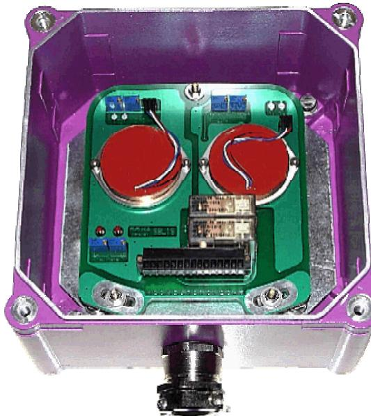
**Sensor box for use in particularly harsh operating conditions containing two sensors, one signal conditioner with 4...20mA output, one signal conditioner with 0...5V output and two safety relays for threshold monitoring**
