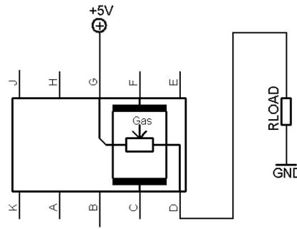
MiCS-2614 with measurement circuit (top view)
