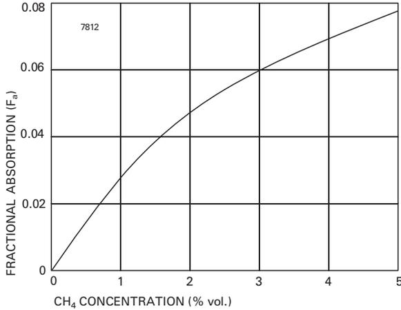
**Fig. 2** Typical Sensitivity to 0 to 5% vol.  $CH_4$
