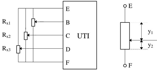
Figure 16. Connection of potentiometers to the UTI.
