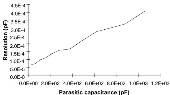
Figure 4 The resolution after the calculation required for the three-signal technique versus the parasitic capacitance  $C_p$ . The measurement range equals 0 - 2 pF.
