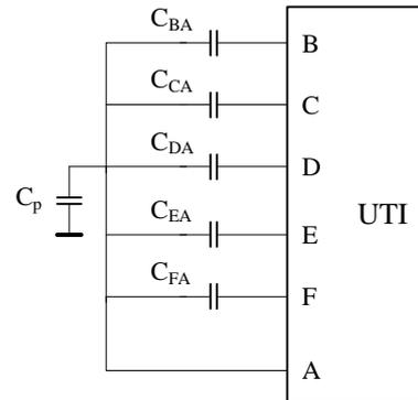
Figure 6. Connection of capacitors to the UTI.
