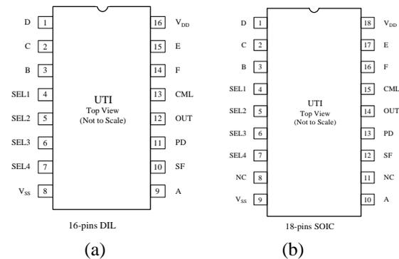
Figure 1 Pin configuration.
