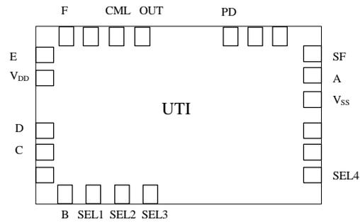
Figure 17 The pad configuration of UTI chip.
