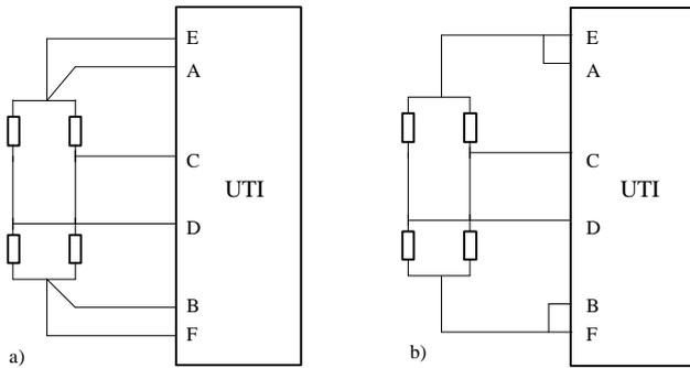
Figure 13. Connection of the resistive bridge to the UTI for the Ub2 mode in a 4-wire setup (a) and a 2-wire setup (b).
