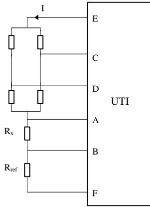
Figure 15. Connections of the sensors to the UTI.
