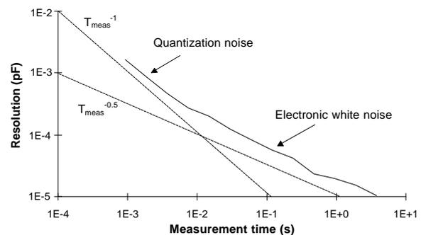
Figure 3 The resolution after the calculation required for the three-signal technique versus the total measurement time. The measurement range equals 0 - 2 pF and  $C_p = 50 \text{ pF}$  (see Figure 7).
