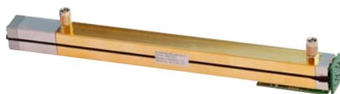
Infrared gas sensor using dual beam technology with measurement and reference channel for use in analytical devices and process control applications. Integrated evaluation electronics for drift and temperature compensation. Robust aluminium cuvette with gas line connectors.
