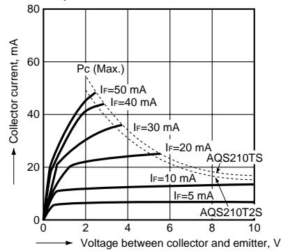
**4-2. Collector current vs. voltage between collector and emitter characteristics ( $I_C-V_{CE}$ )**
