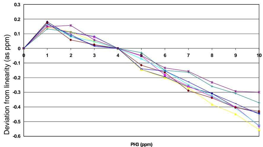
Figure 4 shows variation from linearity to 10ppm. Software correction between 0 and 0.5ppm can improve overall linearity.
