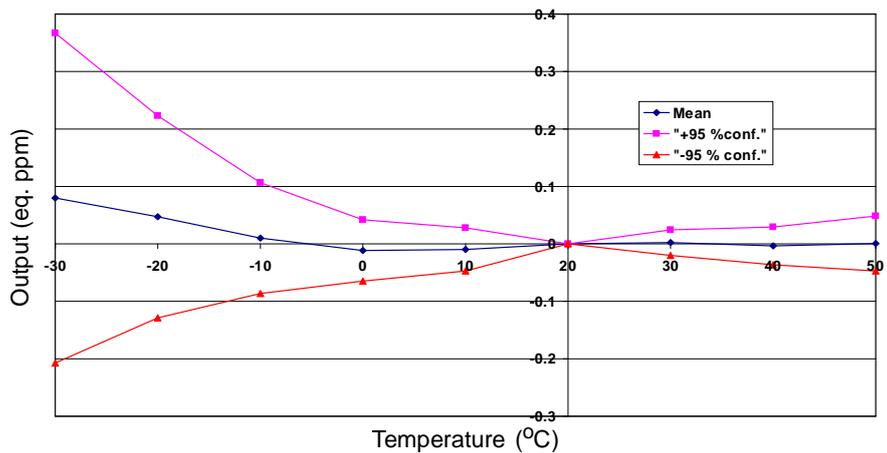
Figure 3 shows the variation in zero output caused by changes in temperature expressed as ppm gas equivalent.
