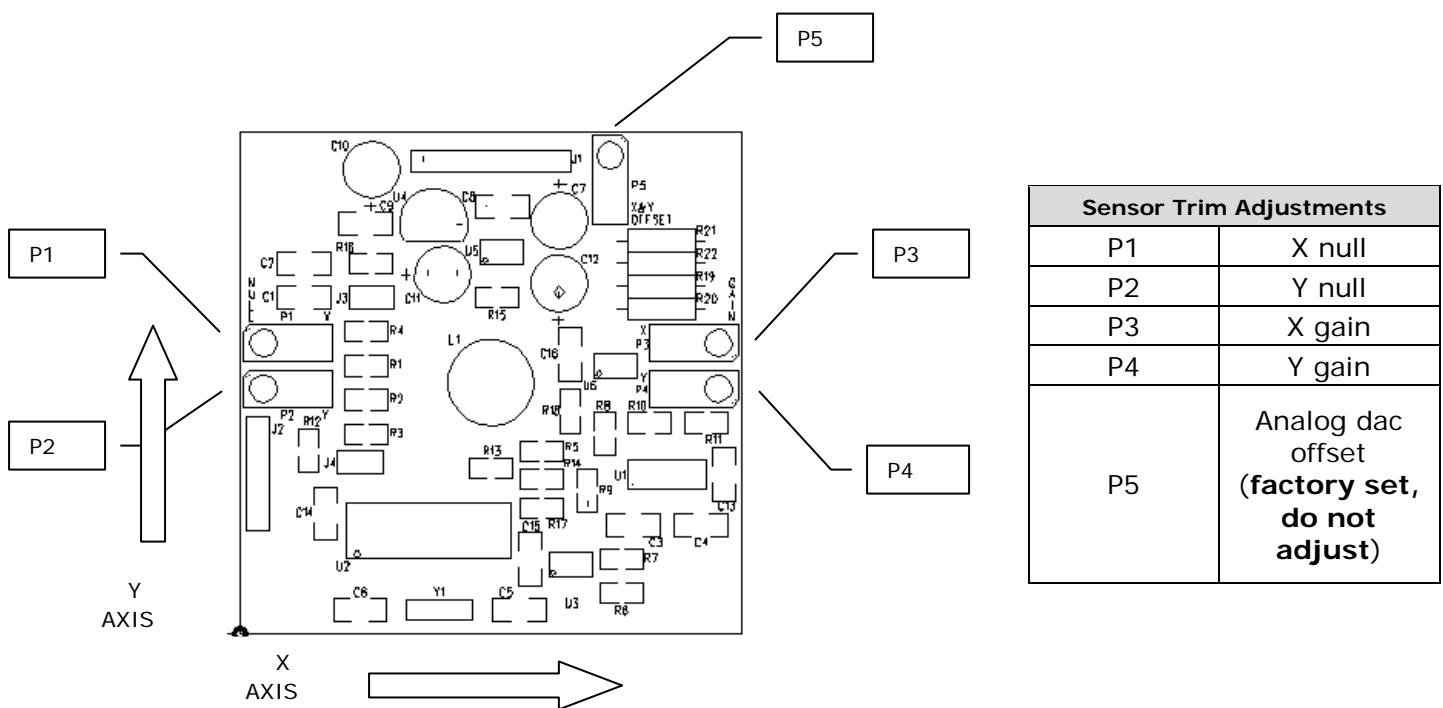
P1 and P2 are offset adjustments for the X and Y analog and digital outputs when the board is in the null or non-tilted position.
