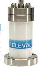
In addition, the 7FCS sensor is specially designed for turn on at ultra high vacuum (UHV). If your application requires ignition in the  $10^{-8}$  Torr range or higher, turn on will occur in less than five seconds. The 7FCS utilizes Double Inverted Magnetron sensor technology combined with a thermionic emitter, which turns on automatically with the cold cathode for five seconds.
