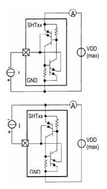
**Figure 4** Latch-up test setup for respective pad and both positive and negative sign. The SHTxx is modeled here as a parasitic thyristor.
