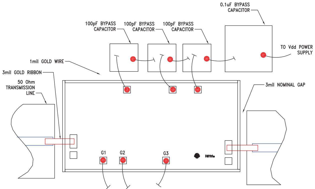
Note: G1, G2 and G3 must be connected to RF/DC ground.
