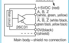
Note: If the transmission distance is long, it should be so considered that the specified voltage occurs at the input portion of the encoder cable end.
