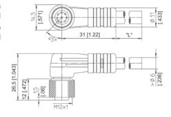
Connector cable for WS® position sensors 8 pin M12 The 8-lead shielded cable is supplied with a mating 8-pin M12 connector at one end and 8 wires at the other end. Available lengths are 2 m, 5 m and 10 m. Wire: cross sectional area 0.25 mm<sup>2</sup>.
