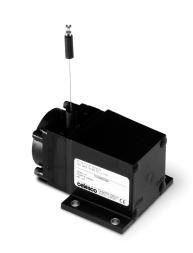
The PT1232, part of our compact line of cable extension transducers, delivers position feedback via RS232 serial communication to your data acquisition or controller system. The PT1232 sends a raw 16-bit position count from 0000 to FFFF (hex). Additionally this device can be set to continuously send data or send data only when polled.
