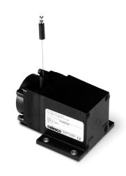
The PT1DN communicates to your PLC over DeviceNET° and provides a precision position feedback signal for full-scale measurement ranges from 2 to 50 inches. Because the PT1DN uses a potentiometer as it's sensing element, the position signal is "absolute" and does not have to be reset to a "home" position upon startup.
