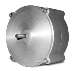
Celesco's model RT9DN communicates rotational position feedback via DeviceNET® to your programmable controller. The heart of this sensor is a precision plastic-hybrid position potentiometer which provides a "absolute" position and does not ever have to be reset to a "home" position after a power loss or planned shutdown.
