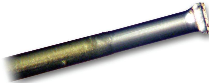
The FOT-HERO is a fiber optic temperature sensor specifically designed for use in Electronic Explosive Device (EED) and HERO-type testing applications. It offers complete immunity to electromagnetic interference and does not emit disturbing signals for the EED circuitry.
