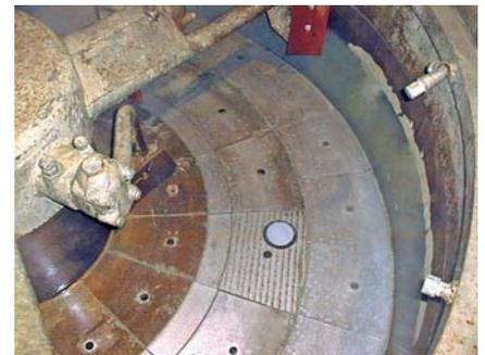
Figure 4: Hydro-Mix sensor
