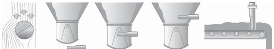
Figure 3: Typical installation positions for a Hydro-Probe II
