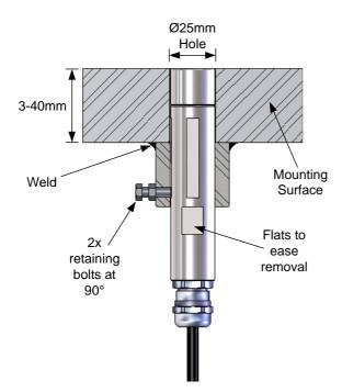
Drill a 25mm diameter hole in the mounting surface and weld the Mounting Collar centrally over it. The Thermo-Tuff is retained by tightening two bolts on to the long flat areas of the sensor.
