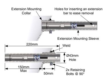
When mounting in a bin or hopper, the Extension Mounting Collar is welded into a 43mm diameter hole. The sensor should be installed into the Extension Mounting Sleeve so that it is flush with the end of the sleeve. It is retained with two grub screws. The Sleeve is then fitted in the Mounting Collar and the retaining bolts used to secure the assembly.
