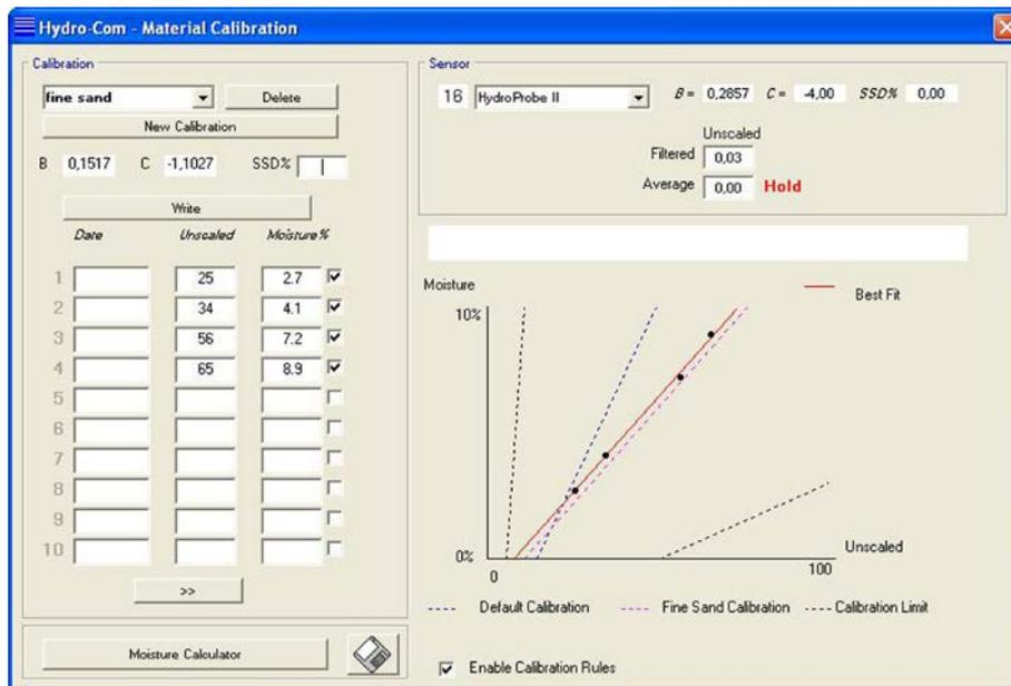
**Figure 5: A multi-point calibration technique is recommended**
