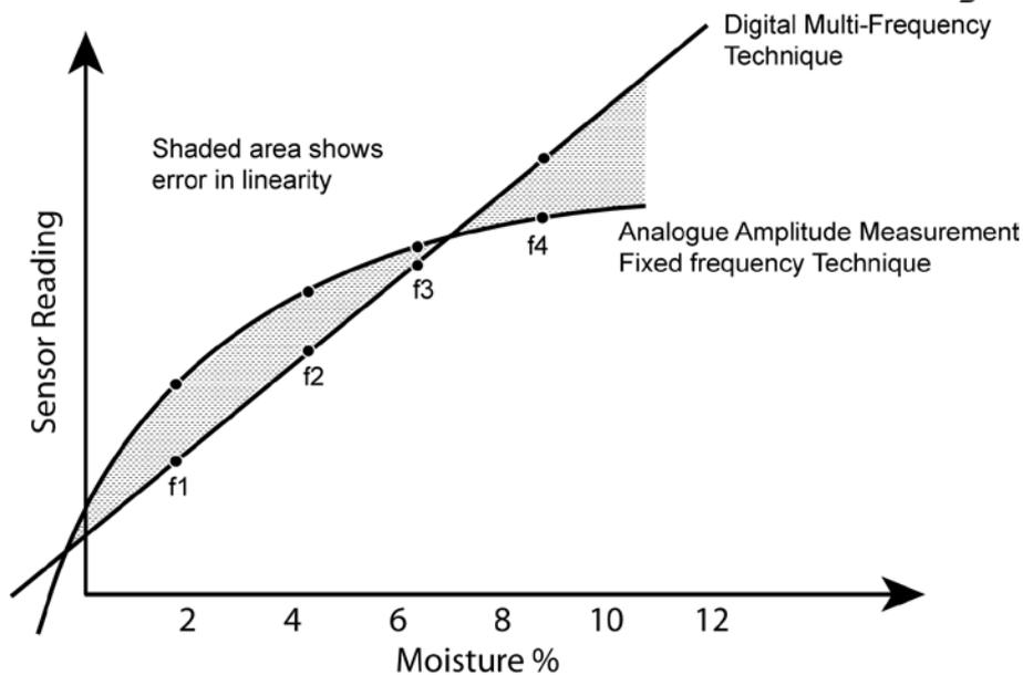
**Figure 3: The effects of a non-linear measurement technique**
