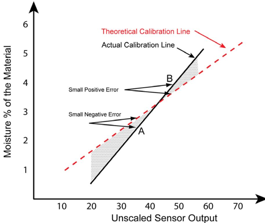
**Figure 4: The effects of assuming a calibration slope**
