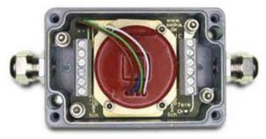
The SB360 integrates the NG360 (360° sensor) with an RS485 data interface - enabling multiple inclinometers to be linked together under harsh operating conditions.
