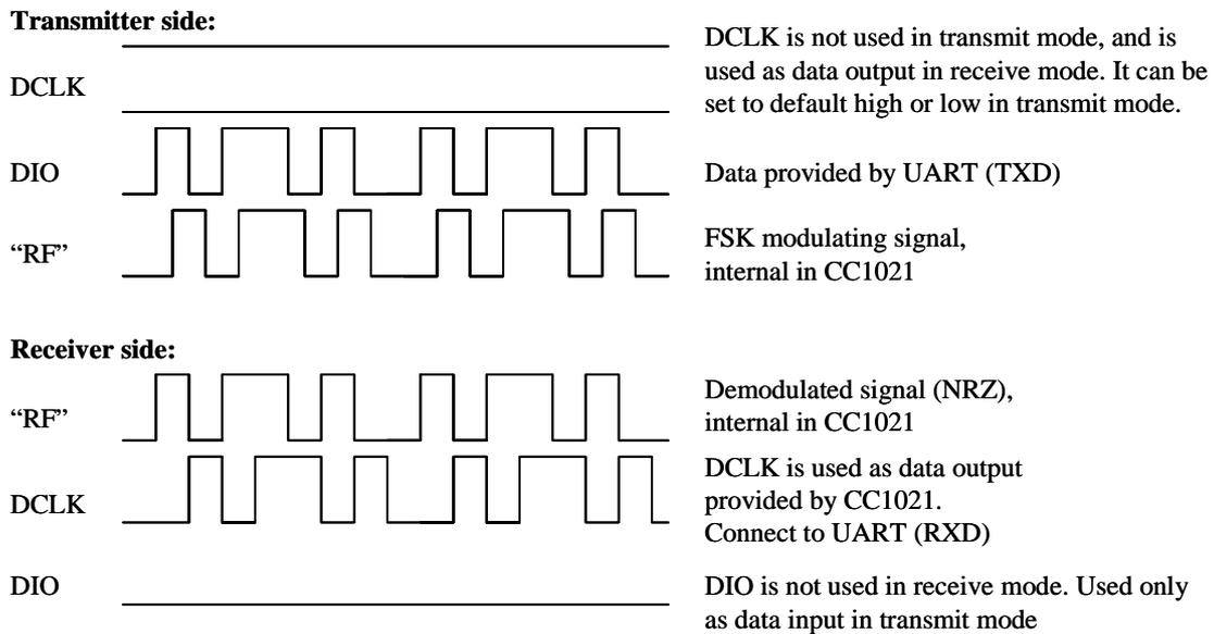
Figure 11. Transparent Asynchronous UART mode ( $SEP\_DI\_DO = 1$ )
