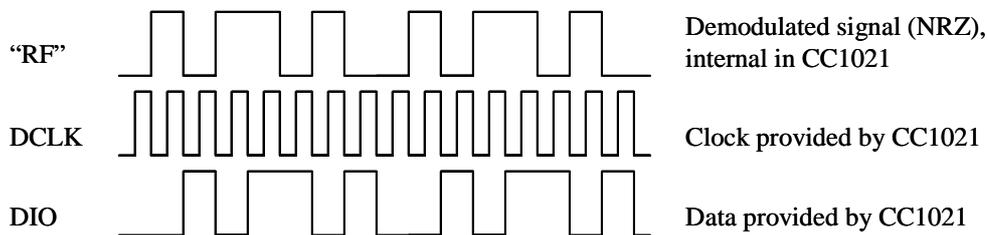
Figure 9. Synchronous NRZ mode ( $SEP\_DI\_DO = 0$ )
