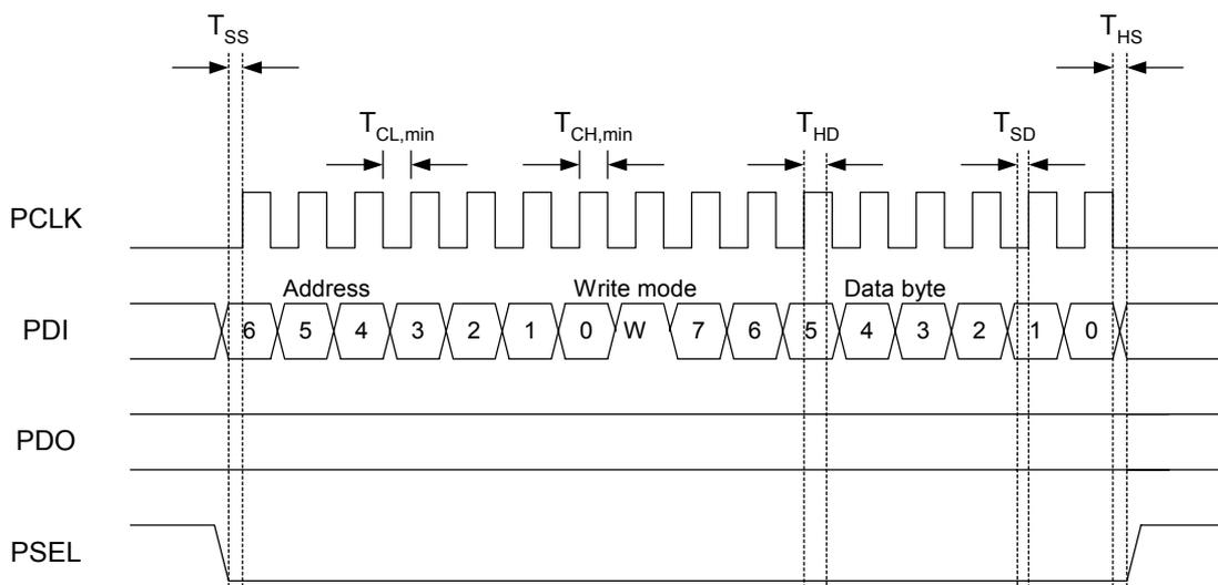
Figure 7. Configuration registers write operation
