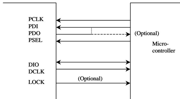
Figure 6. Microcontroller interface
