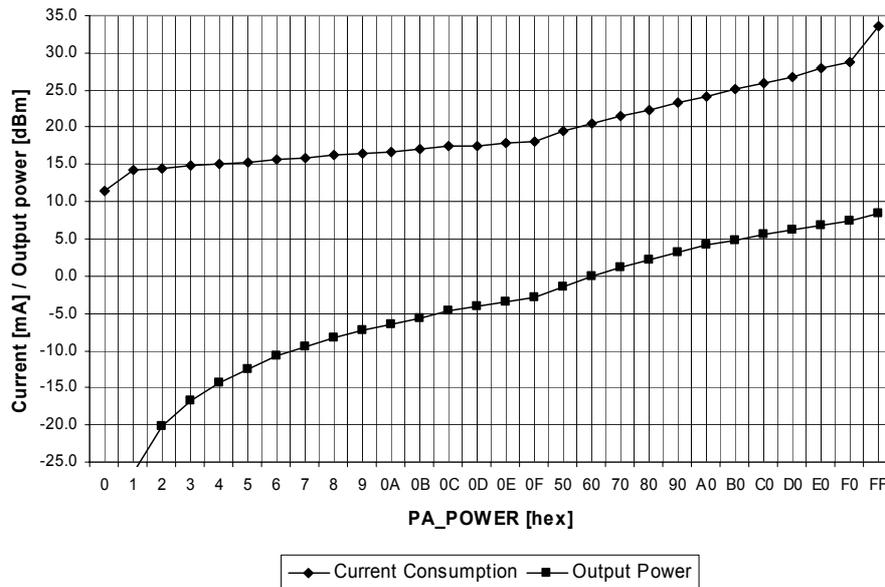
Figure 24. Typical output power and current consumption, 868 MHz
