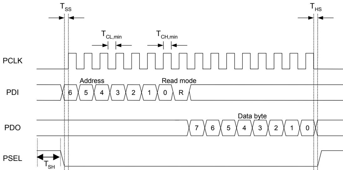
Figure 8. Configuration registers read operation
