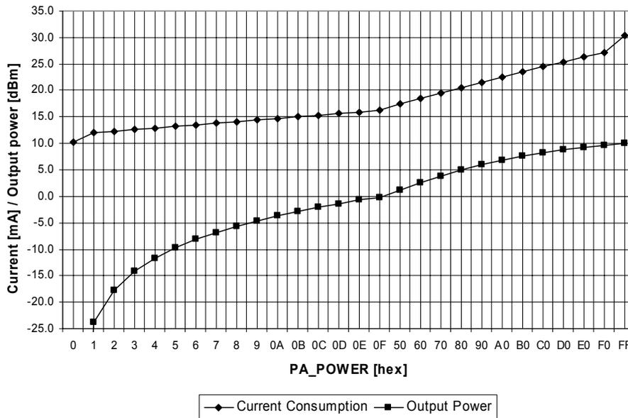
Figure 23. Typical output power and current consumption, 433 MHz
