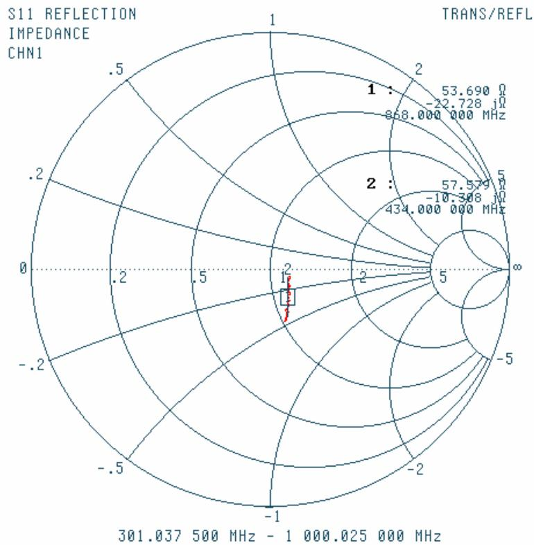
Figure 26. Typical LNA input impedance, 200 – 1000 MHz
