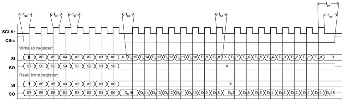
Figure 6. SPI timing diagram
