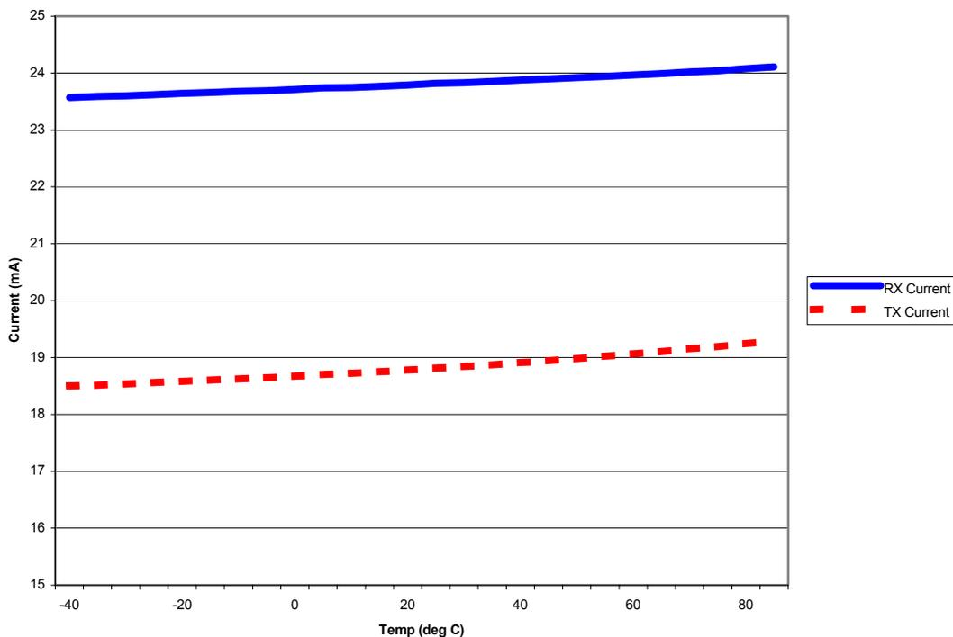
**Figure 24 Typical RX and TX current vs. temperature**
