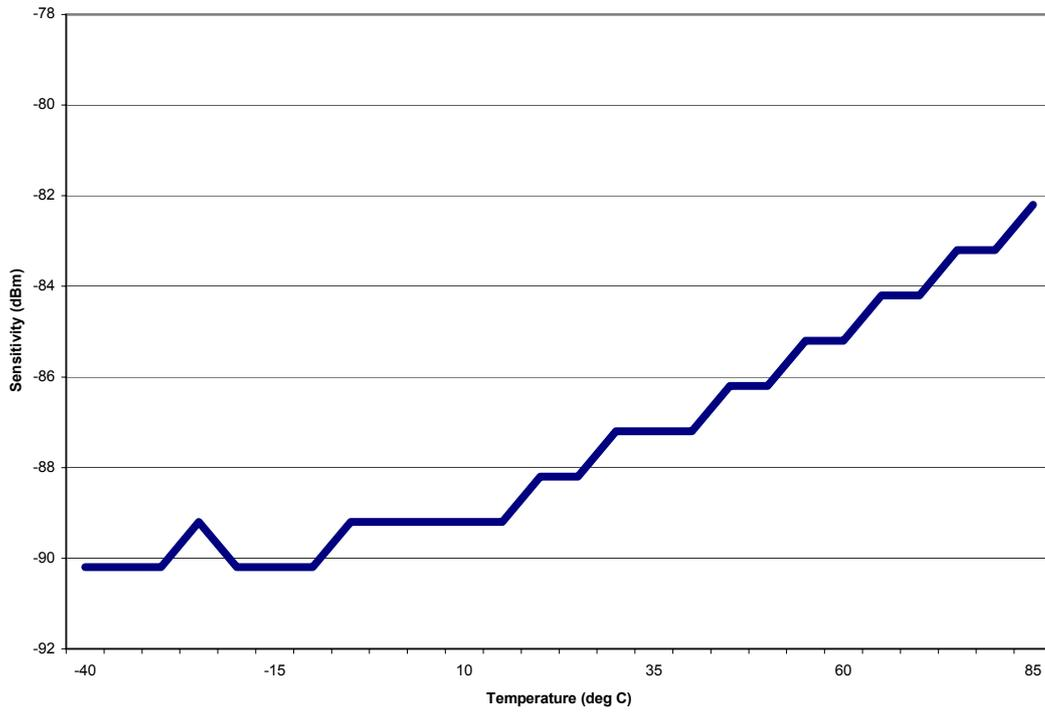
Figure 27 Typical 1 Mbps sensitivity vs. temperature
