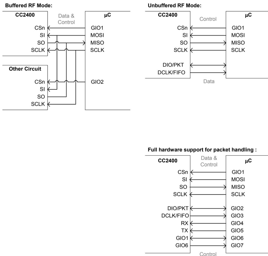
**Figure 8. Microcontroller interface**
