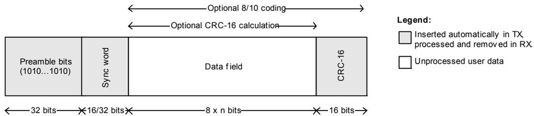
**Figure 11. Packet format details (with recommended lengths of preamble and synchronization word)**
