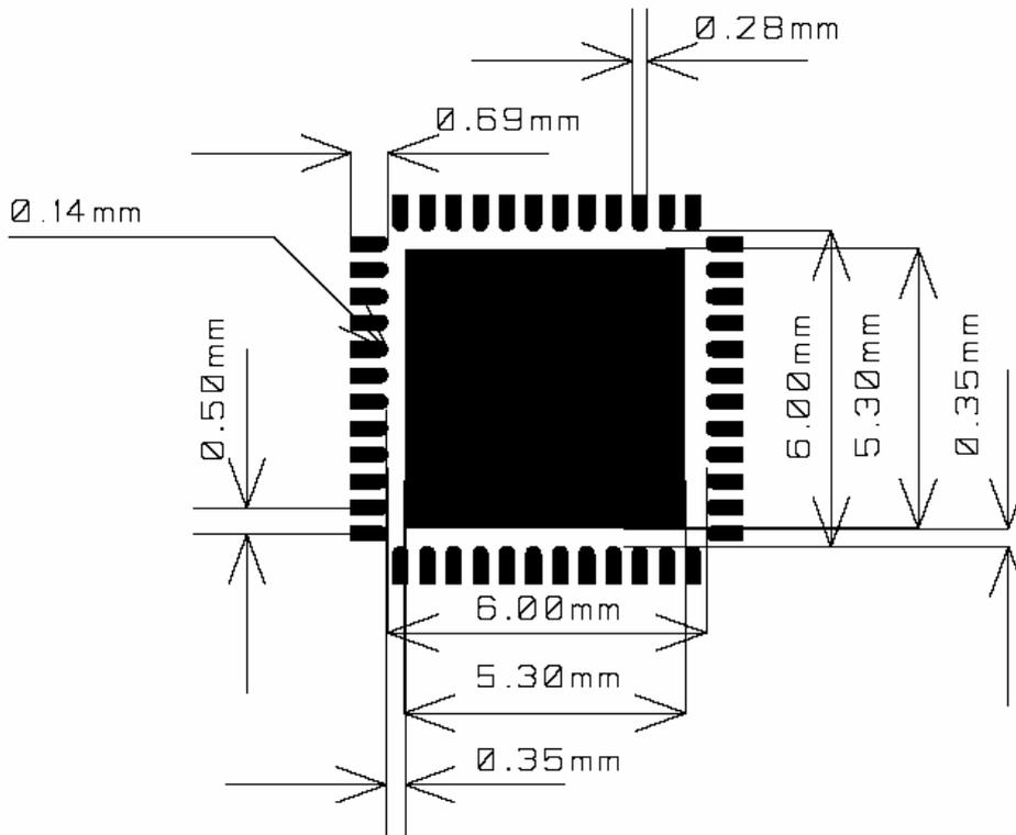
Note: The figure is an illustration only and not to scale. There are nine 14 mil diameter via holes distributed symmetrically in the ground pad under the package. See also the CC2400EM reference design.
