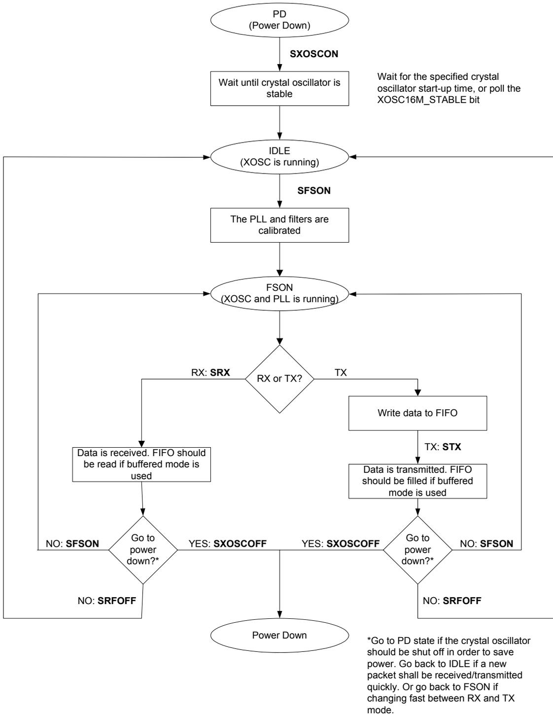
**Figure 17. Sequence for activating RX or TX mode**
