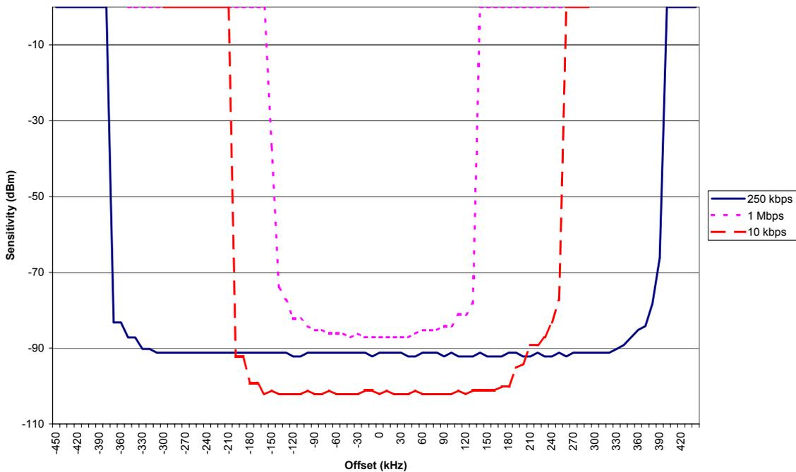
**Figure 19. Sensitivity as a function of frequency offset**
