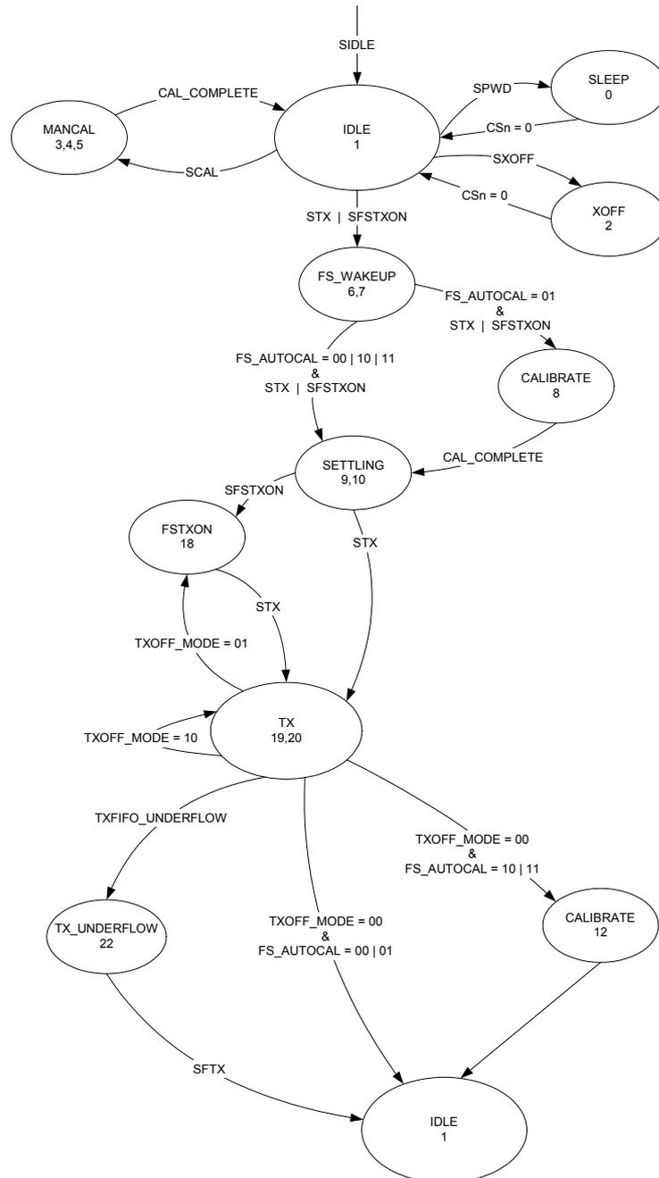
Figure 10: Radio Control State Diagram
