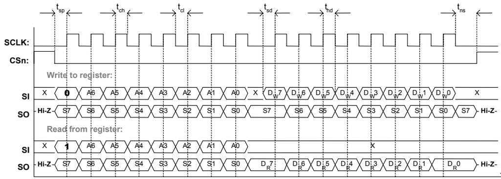
Figure 6: Configuration registers write and read operations
