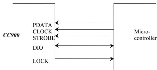
**Figure 6. Microcontroller interface.**
