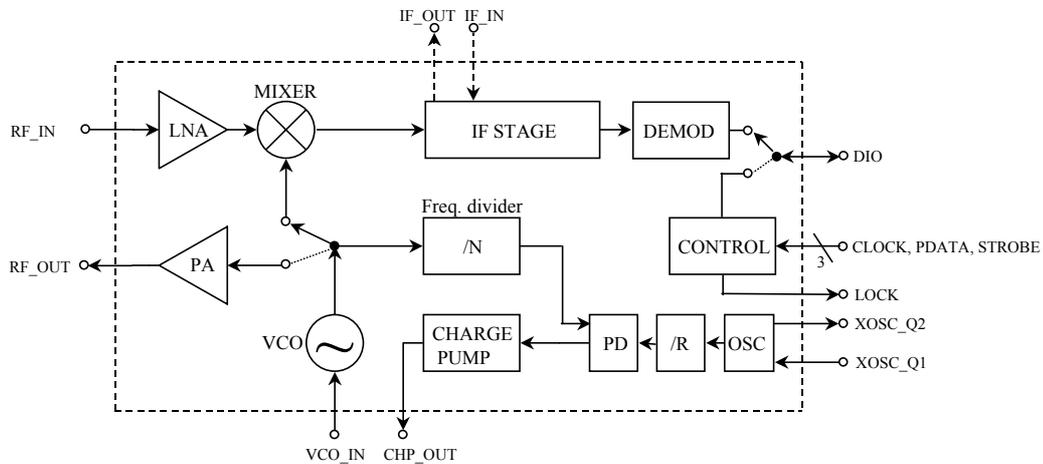
Figure 1. Simplified block diagram of the **CC900**.
