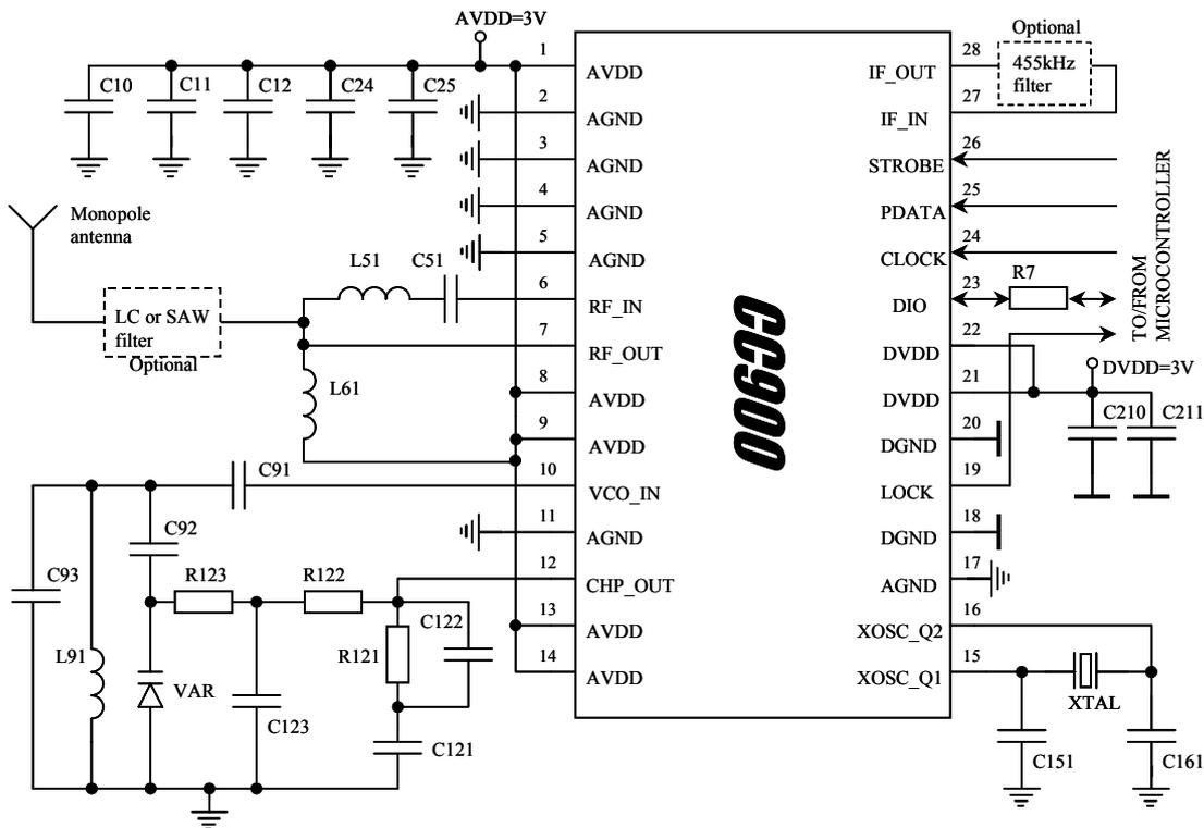
Figure 7. Typical **CC900** application for 869.000 MHz operation.
