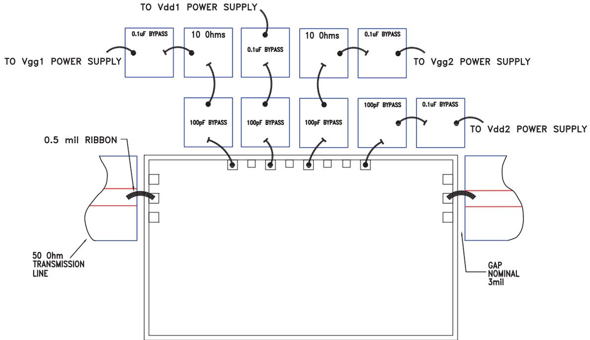
Note 1: Bypass caps should be 100 pF ceramic (single-layer) placed no further than 30 mils from the amplifier
