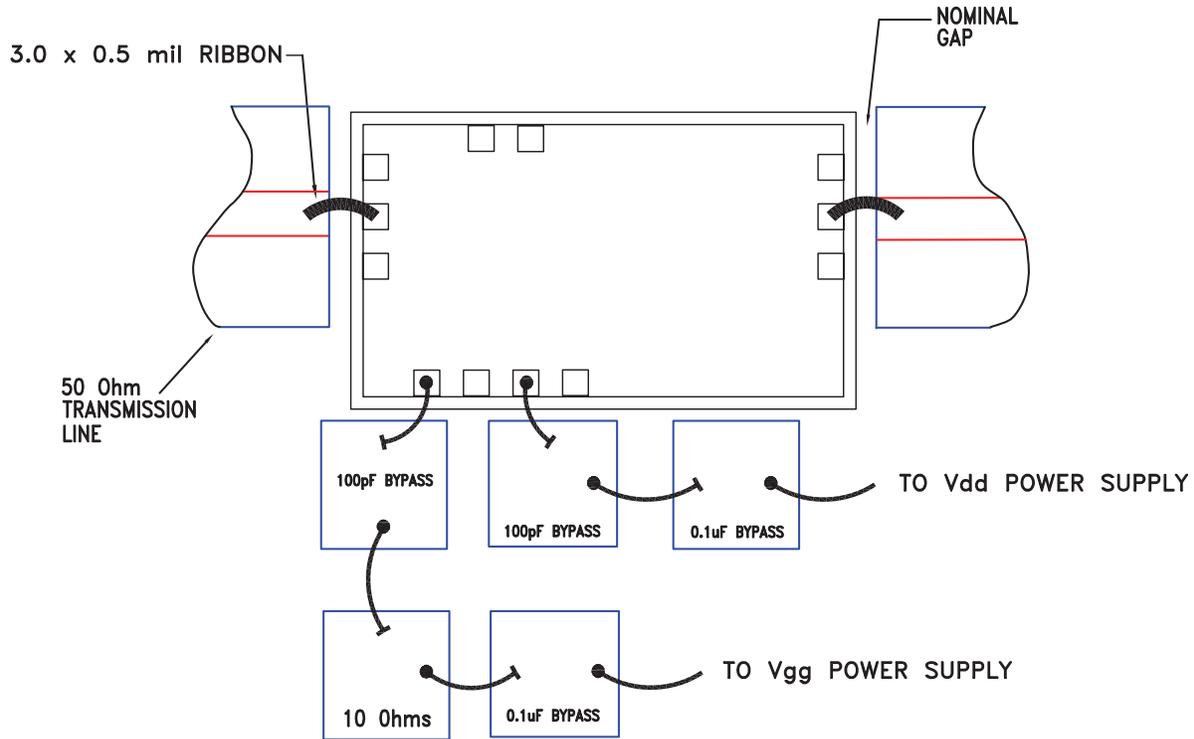
Note 1: Bypass caps should be 100 pF (approximately) ceramic (single-layer) placed no farther than 30 mils from the amplifier.
