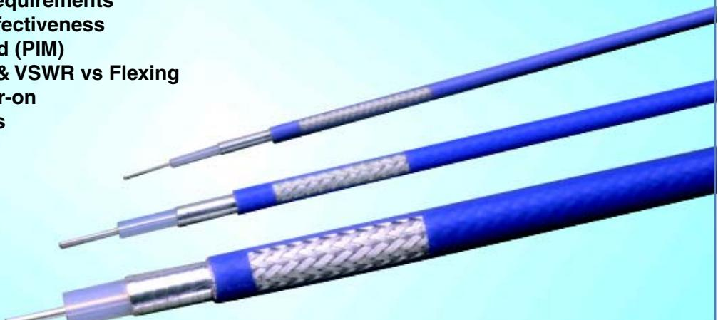
**TFlex** employs a thin helical wrap of silver plated copper tape and overall braid sized such that standard solder-on connectors can be used.
