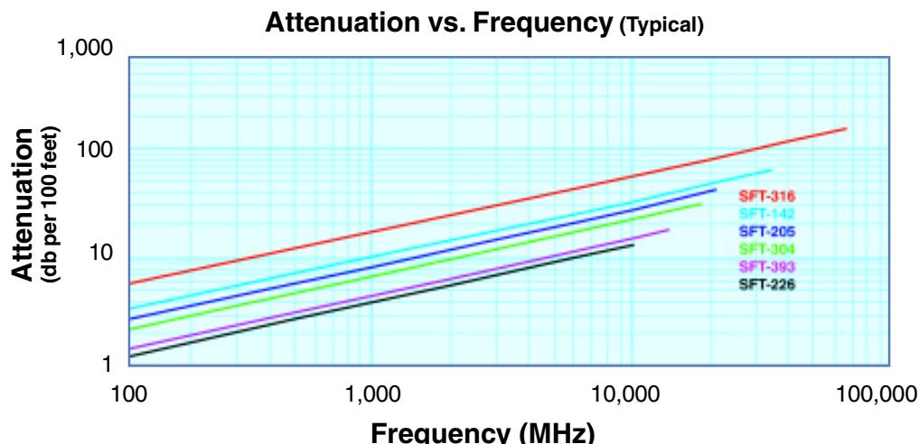
Attenuation at Any Frequency = [ k1 x  $\sqrt{F\text{MHz}}$  ] + [ k2 x F<sub>MHz</sub> ]; dB per 100 feet
