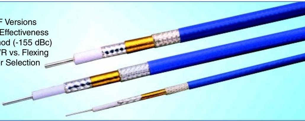
**StripFlex-II** cables provide the ultimate performance in a flexible cable. The low density PTFE tape dielectric provides the lowest dielectric loss of any practical dielectric and silver plated conductors make these the ideal choice for microwave applications and other commercial and military interconnect systems.
