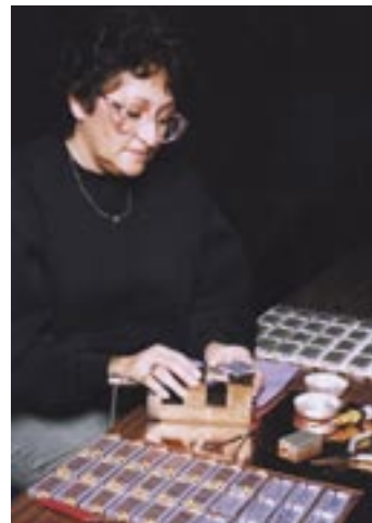
A production associate assembles a 2 GHz filter for a leading test equipment manufacturer.
