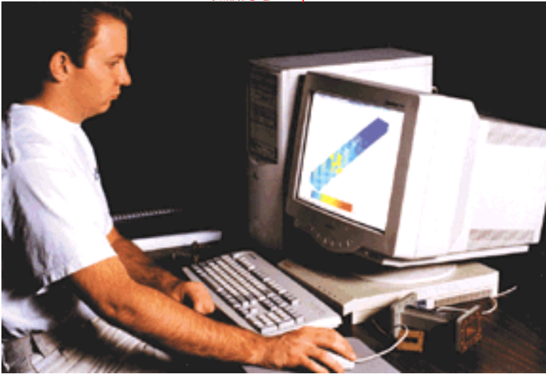
Finite element analysis software allows the modeling of complex waveguide structures.
