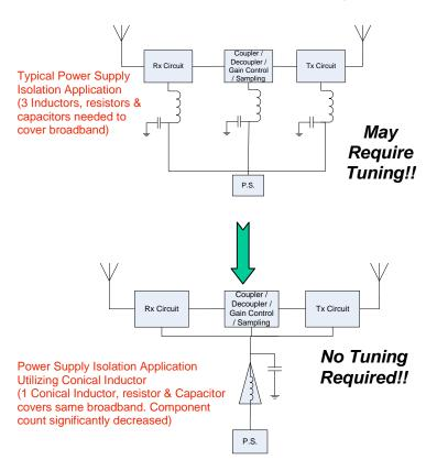
Note: Other sub-assembly applications include, but not limited to; Oscillators, Fr. Multipliers, Bias Networks, Switches Amplifiers, Fiber Optic Transmitter Receiver Circuits...
