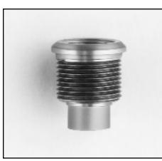
The use of a lossy rod material for the rotor of the tuning element provides a convenient and effective means of trimming the microwave device in a waveguide or cavity. The amount of power absorbed is a function of the depth of insertion of the rod into the waveguide or cavity. Standard models are ideal for frequencies of 1 to 18 GHz.
