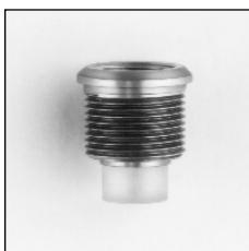
The use of a dielectric rod (instead of a metallic probe) for the tuning element will provide the lowest loss tuning for high frequency applications. When the dielectric rod is introduced into a microwave cavity it has the effect of making the cavity electrically larger, and lowering the resonant frequency. Dielectric tuning elements are excellent for adjusting the frequency of Gunn diode and IMPATT oscillators.
