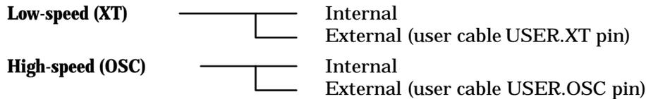
The microcontroller's time-base counter always uses the XT input to generate clock signals for the onboard peripherals. Its CPU, however, offers a choice of clock speeds: XT or OSC.
