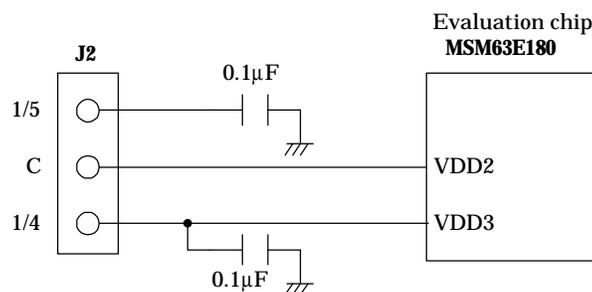
Figure 2-21 Jumper 2 Circuit
