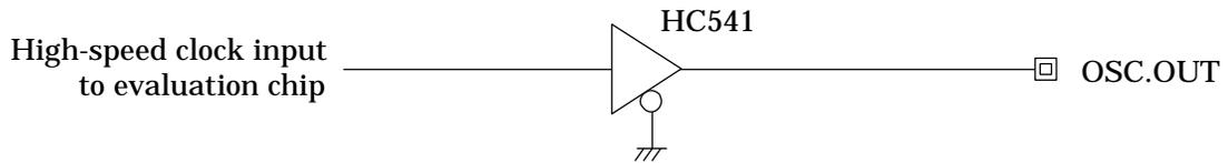
The high-speed clock (OSC.OUT) signal uses the emulator's internal operating voltage (5 V) for its "H" level.
