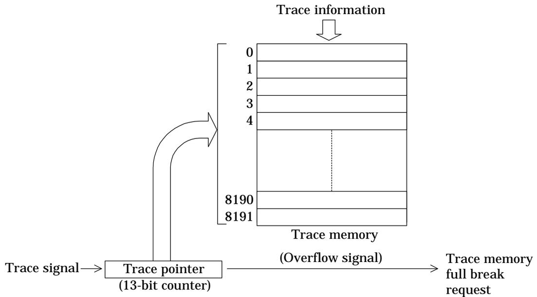
If trace memory full breaks are enabled, overflow during real-time emulation of the trace pointer, a 13-bit counter, produces a break request of this type.
