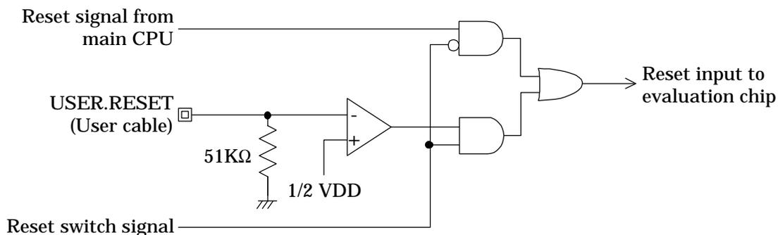
**Figure 2-19 Reset Input**
