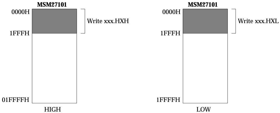
**Figure 2-2 Address Ranges for MSM27101**
