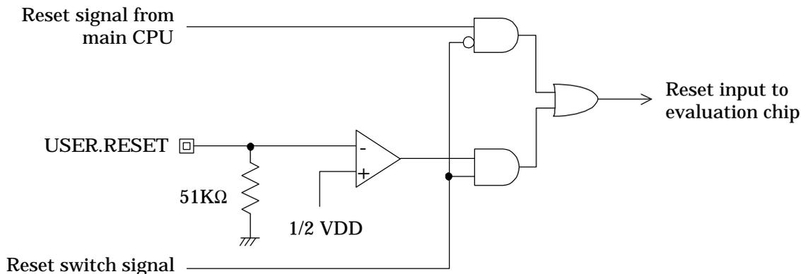
A built-in voltage conversion circuit converts the user cable reset (USER.RESET) input to the internal “H” level from VDD, the positive power supply voltage (0.9 to 5 V).
