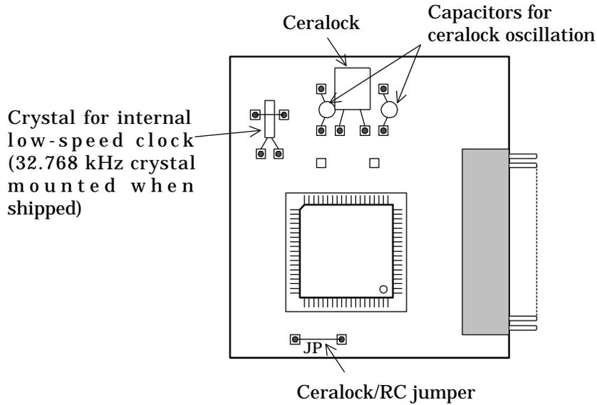
To use RC oscillation, install an ROS resistor with the value given in the user's manual for the microcontroller.
