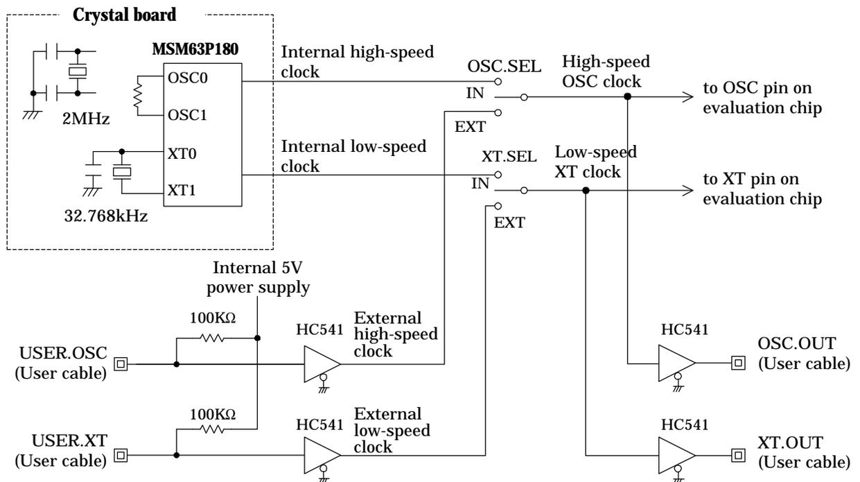
Figure 2-17 Clock Circuits
