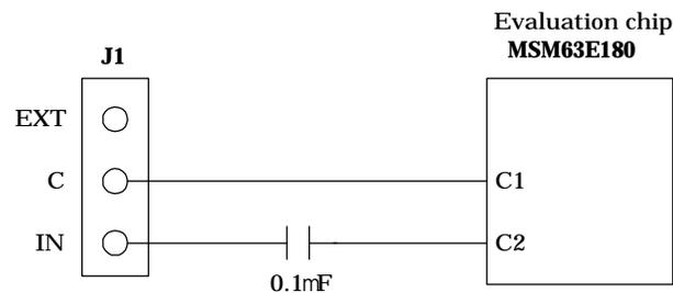
Figure 2-20 Jumper 1 Circuit
