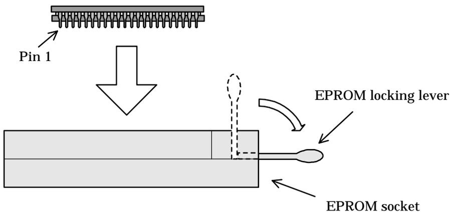
The sockets accept the following EPROM types. Note how the position of pin 1 differs for each type.
