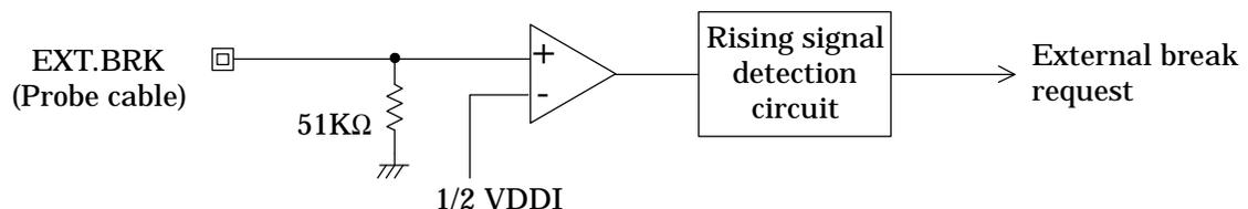
A built-in voltage conversion circuit converts the break (EXT.BRK) input level of VDDI, the port interface power supply voltage (0.9 to 5 V), to the internal “H” level.
