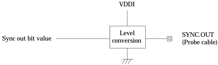
A built-in voltage conversion circuit converts the sync out (SYNC.OUT) signal “H” level to VDDI, the port interface power supply voltage (0.9 to 5 V), for output.
