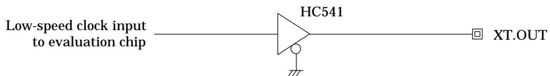
The high-speed clock (XT.OUT) signal uses the emulator's internal operating voltage (5 V) for its "H" level.
