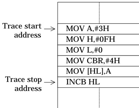
Tracing covers from the MOV A,#3H instruction at the start address through to the MOV [HL],A instruction preceding the stop address.
