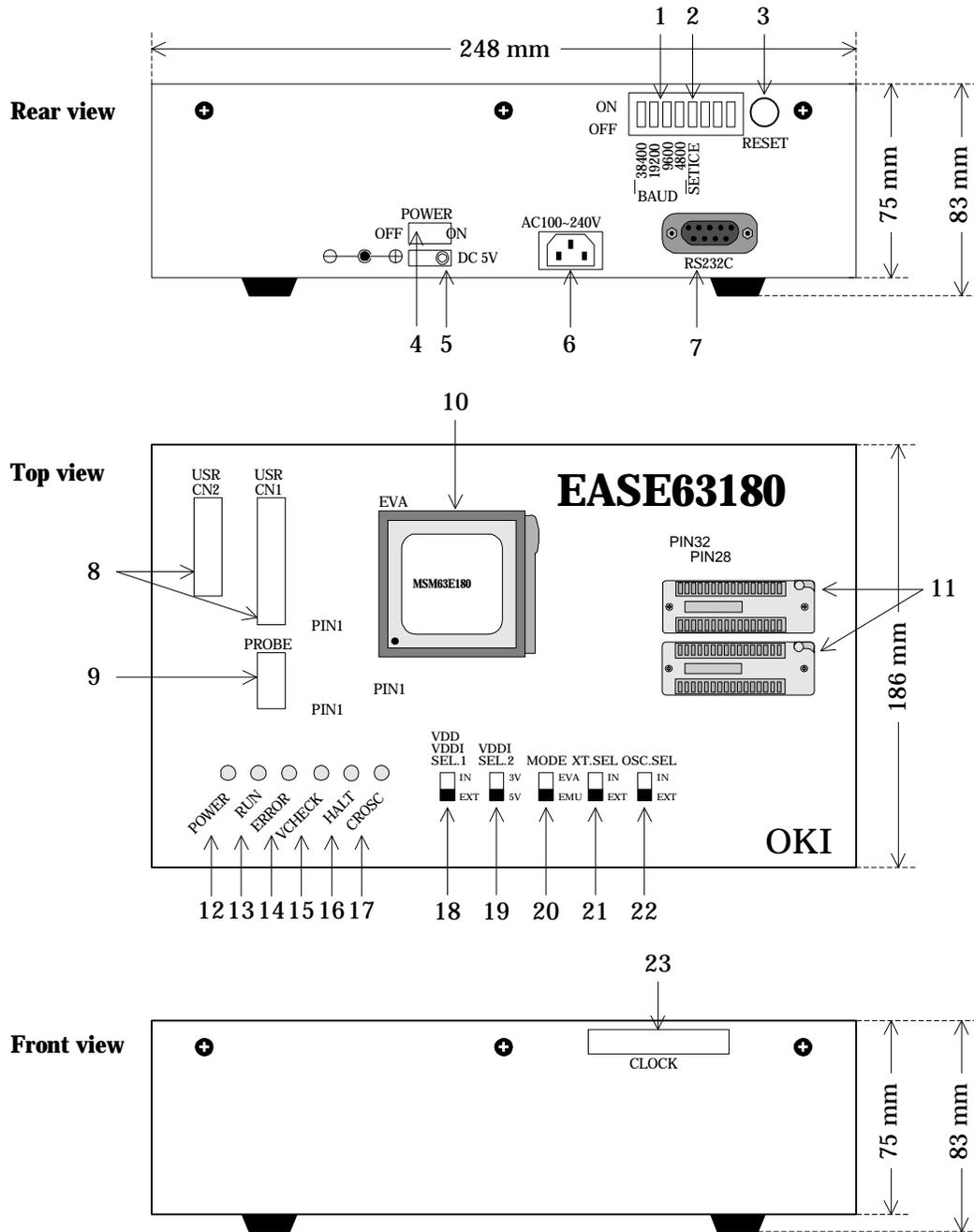
**1. Baud rate switches (BAUD)**
