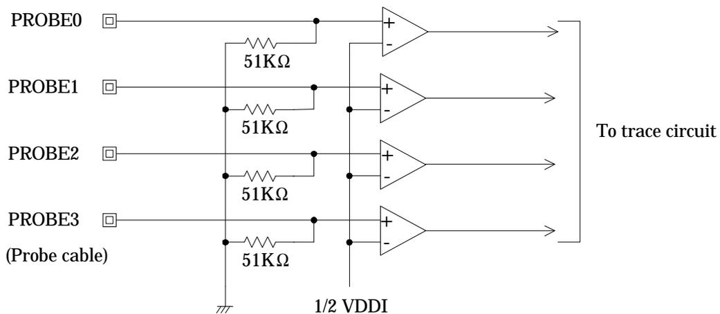
Built-in voltage conversion circuits convert the trace (PROBE0 to PROBE3) inputs to the internal "H" level from VDDI, the port interface power supply voltage (0.9 to 5 V).
