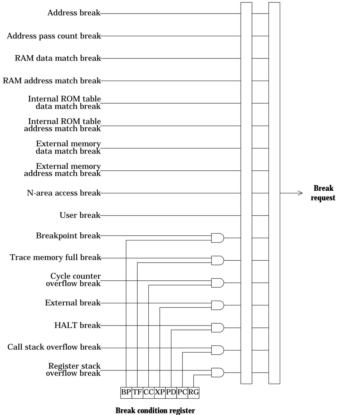
**Figure 2-3 From Break Condition to Break Request**
