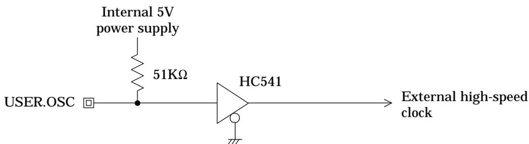
The user cable high-speed clock (USER.OSC) input uses the emulator's internal operating voltage (5V) for its “H” level.
