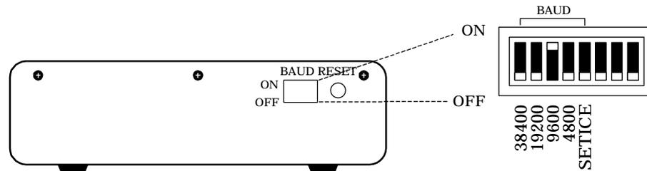
Figure 2-22 BAUD Switch
