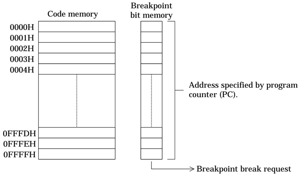
If these breaks are enabled, execution of the instruction at that address produces a break request of this type.
