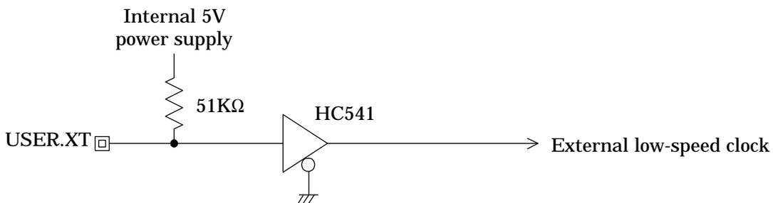
The user cable low-speed clock (USER.XT) input uses the emulator's internal operating voltage (5 V) for its “H” level.
