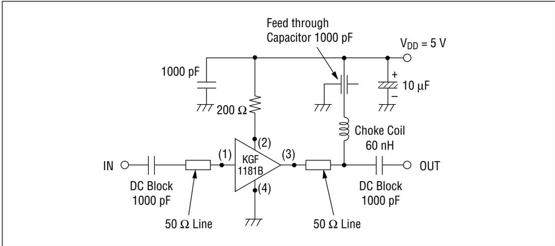
**Test Circuit Board for KGF 1181B**
