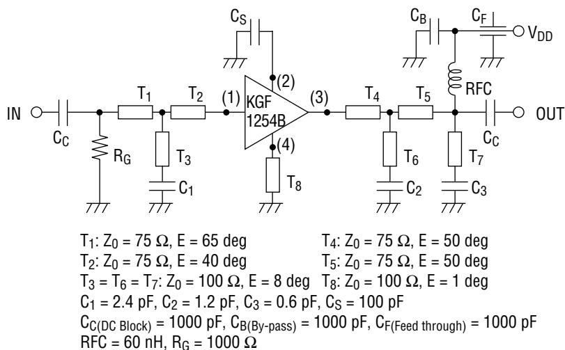
**Test Circuit and Bias Configuration for KGF1254B at 1.9 GHz**
