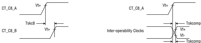
Figure 16. Clock Skew Requirements
