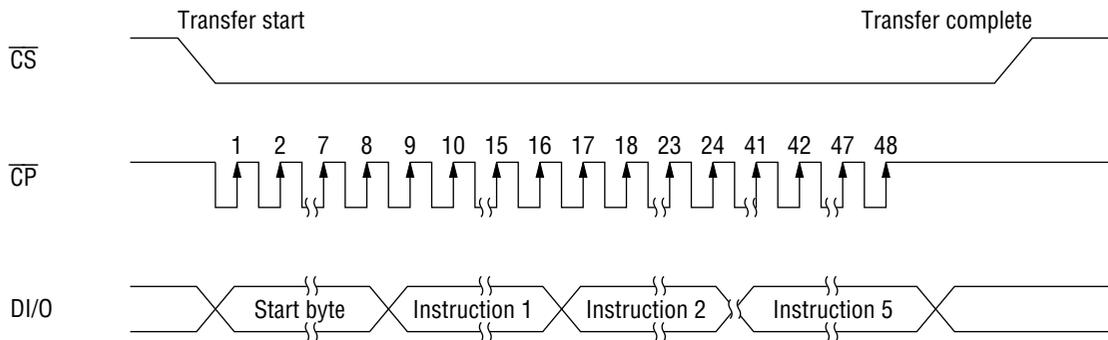
**Clock Synchronous Serial Continuous Data Transfer Example (READ)**
