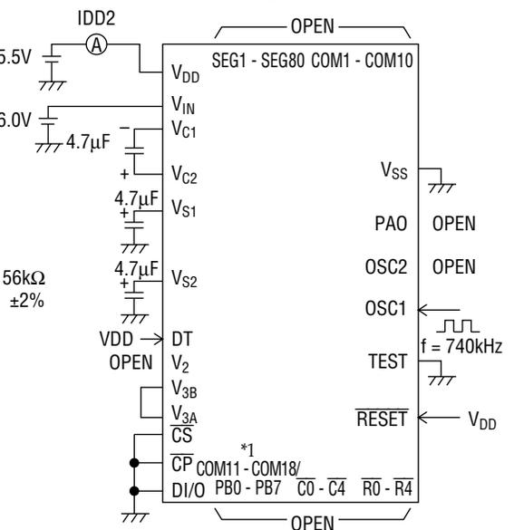
\*1: PB0 - PB7 for ML9090-01, and COM11 - COM18 for ML9090-02
