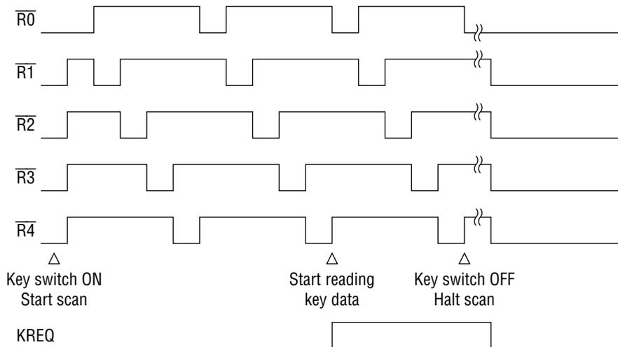
Note 1: Pressing three or more key switches simultaneously may result in incorrect recognition (a switch that was not pressed may be recognized as a switch that was pressed). Therefore, if it is necessary to recognize three or more pressed switches, connect a diode in series with each switch. If three or more pressed switches are not to be recognized, data should be ignored if there are three or more "1s" in the key data that is read by software.
