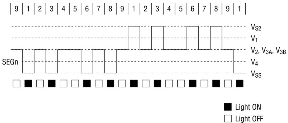
Liquid Crystal Driving Waveform Example
