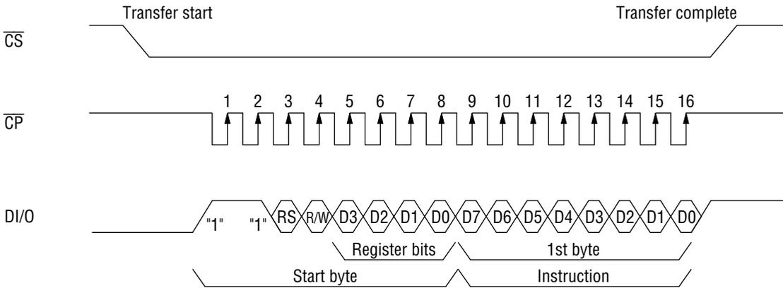
**Clock Synchronous Serial Continuous Data Transfer Example (WRITE)**
