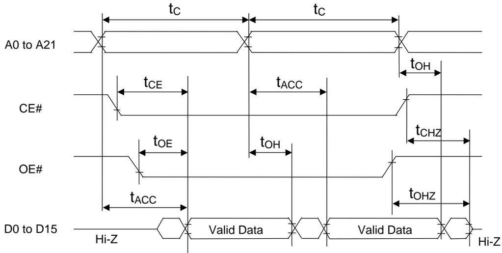
**8-Bit Read Mode (BYTE# = V<sub>IL</sub>)**
